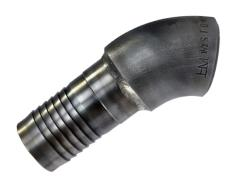
The EBB is a ready to use 45° elbow terminated with a genuine DMIC hose barb. This adapter was developed in response to customer requests for an easy way to terminate Sch. 40 pipe runs with a hose barb. Also offered in **BBE** 90° version: See pg. 15
