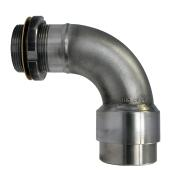
The SNE is ideal for placement of inlet valves in mechanically rigid flooded suction positions. Internal thread/socket weld allows mounting of strainer or baffle pipe. External thread with swivel feature permits perfect alignment of shutoff valve.
