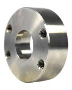
The FCM is a flat weld SAE 4-Bolt Companion Flange optimized for use as a reservoir outlet connection. An internal thread provides a mounting point for strainer or baffle tube.
