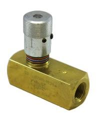
Flow-regulating, brass body flow control valves with a built-in 5 psi check valve. Provides regulated flow in one direction and free flow in the opposite direction.
