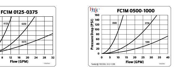
Note: [2] Flow characteristics shown are nominal values only. Actual results may differ depending on fluid viscosity, temperature, and port connection. This valve series is factory sealed and disassembly will destroy the valve and void the warranty. Due to our policy of continual product improvement, the specifications in this catalog may change without notice. When designing by spec, please request a certified print.
