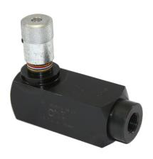
Flow-regulating needle valves with a built-in 5 psi check valve. Provides metered flow in one direction and free flow in the opposite direction. Flow rate is maintained within 5% in the event of upstream or downstream pressure fluctuations.
