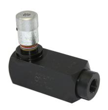
Flow-regulating needle valves provide metered flow in both directions. Flow rate is maintained within 5% in the event of upstream or downstream pressure fluctuations.
